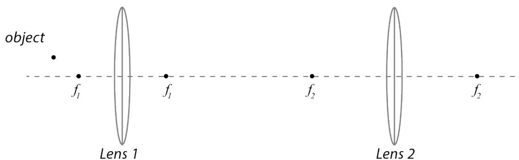
4. Think of lens 1 as the objective lens and lens 2 as the eyepiece lens of a microscope. Does the eyepiece lens form an image that could be viewed on a screen? If so, where should the screen be placed? If not, is it possible to adjust lens 2 so that its image could be viewed on a screen?
